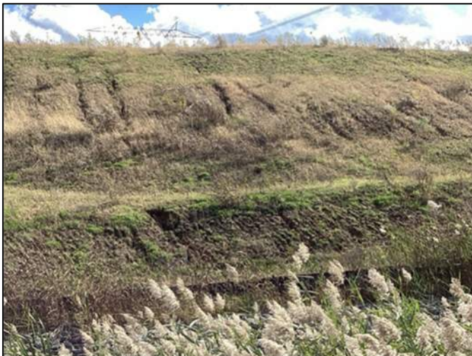
Photo 66, Point 66 Erosion rills on stockpile located north of Northeast Sedimentation Basin.
